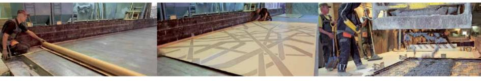
The casting is prepared by cleaning the mould and cutting the membrane according to the element drawings. It is recommendable to use a vacuum table. The membrane is spread out on the clean mould table with the retardered side facing the concrete.
