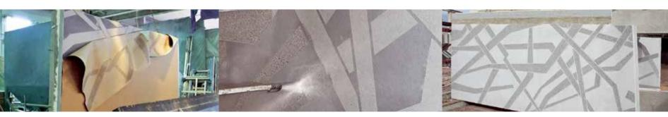
The element is transported to the washing area and the membrane comes off.
