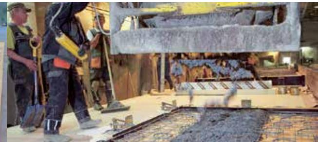
The casting is prepared by cleaning the mould and cutting the paper according to the element drawings. It is recommendable to use a vacuum table.
